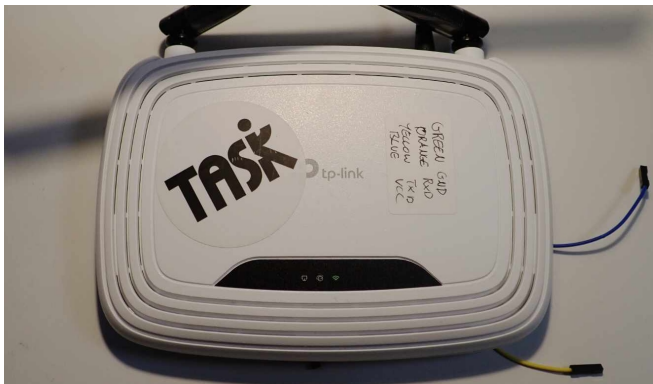
Figure 3: UART cable colors labeled
